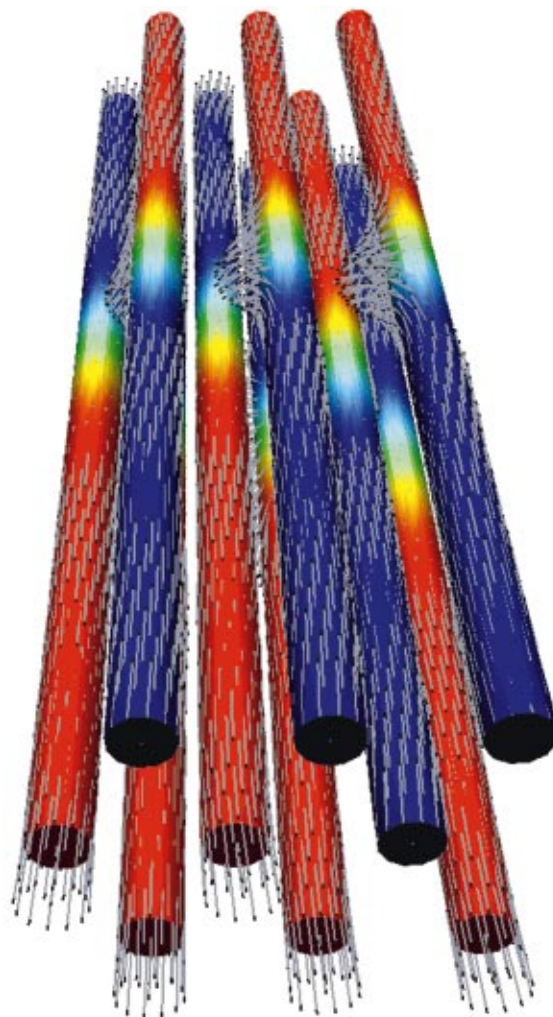
FIG. 10. (Color) Zero field magnetization state of an array of nine nanowires after saturation perpendicular to the wire axis. The magnetic configuration of the wires is split in two domains.
