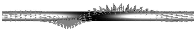
FIG. 3. A 360^\circ wall may also be found as a metastable magnetization distribution.
