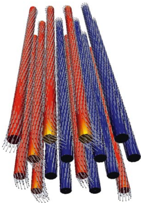
FIG. 8. (Color) Perspective view on 16 nanowires near the coercive field. The colors represent the z component of the magnetization: The blue wires have switched while the red wires are magnetized in their original state. The small yellow regions indicate the onset of magnetization reversal.
